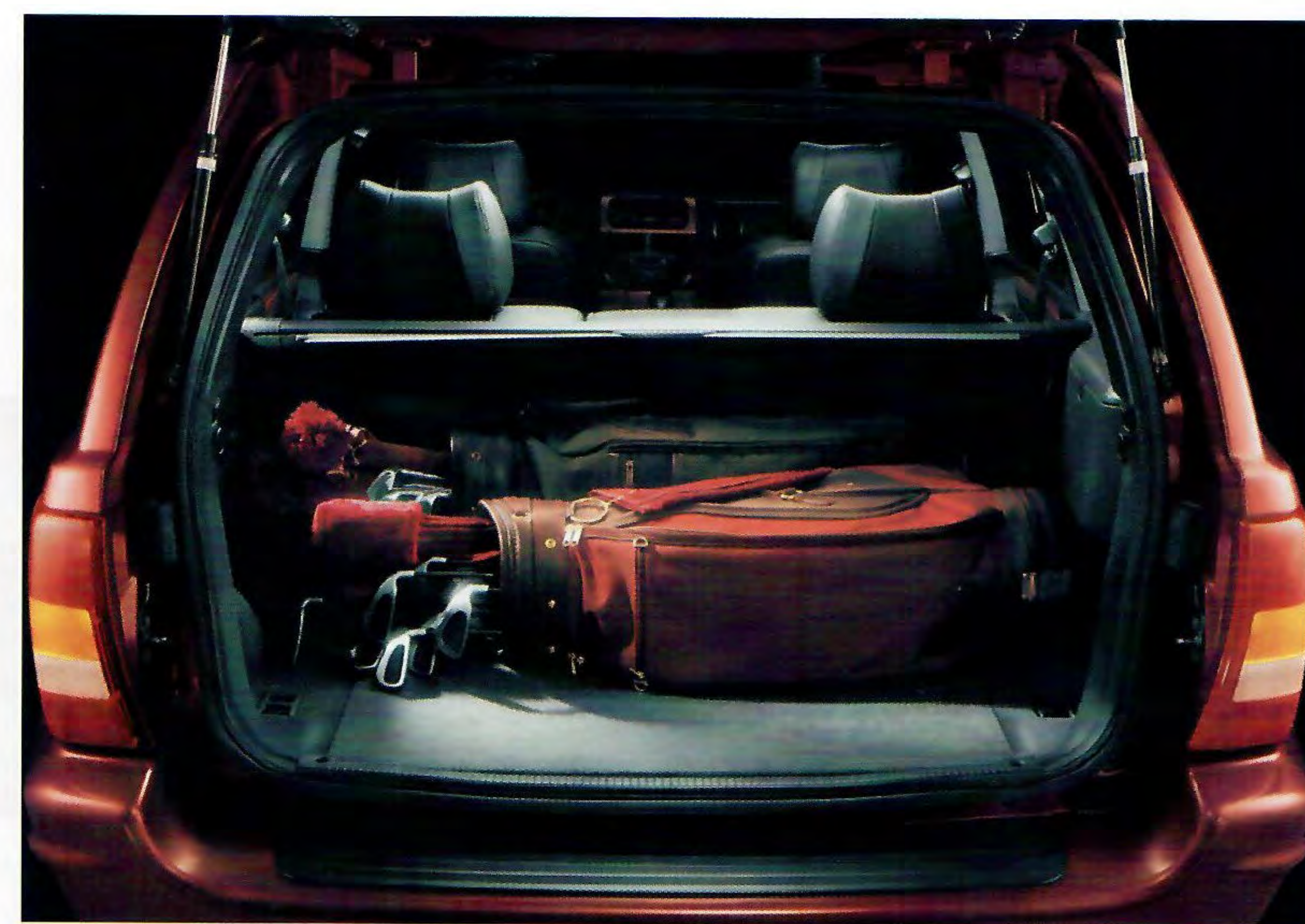
With the rear seats up, Grand Cherokee offers 39.0 cubic feet of cargo space. Fold them down and 72.3 cubic feet are available. And with the spare tire now under the rear load floor, that space is more usable than ever for your favorite gear or golf clubs.
